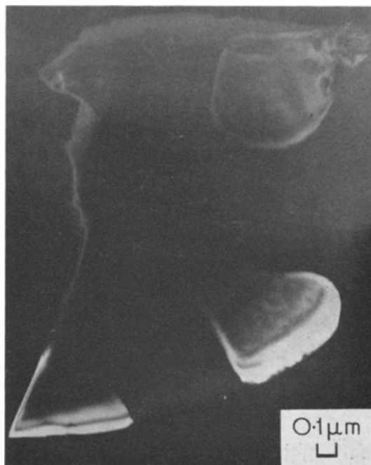
Figure 4 Dark field image, showing three large precipitate grains in a matrix of \alpha\text{-LiFeO}_2 , after heating at 1100° C for 65 h.
